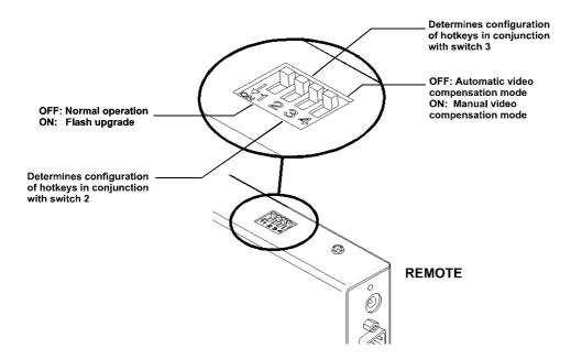
Note: When shipped, all switches are set in the OFF positions and this will produce normal operation.
